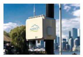
AirSENCE has been developed in collaboration with the Southern Ontario Centre for Atmospheric Aerosol Research (SOCAAR) at the University of Toronto, a leading-edge research institute. It incorporates a fast-response, multi-parameter sensor array and robust machine learning-based signal processing and data fusion to provide an Industrial Internet of Things (IIoT) network for real-time, 24/7 ambient air monitoring.
